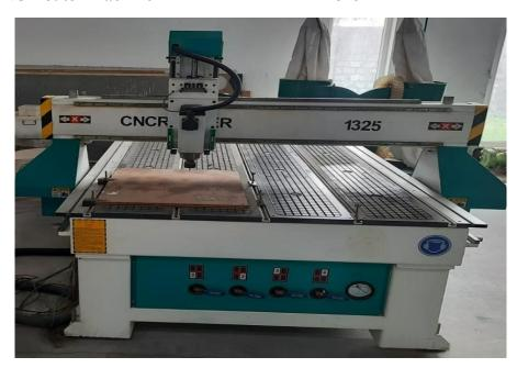
A **computer numerical control** (CNC) **router** is a computer-controlled cutting machine which typically mounts a hand-held router as a spindle which is used for cutting various materials, such as wood, composites, metals, plastics, glass, and foams. CNC routers can perform the tasks of many carpentry shop machines such as the panel saw, the spindle moulder, and the boring machine.
